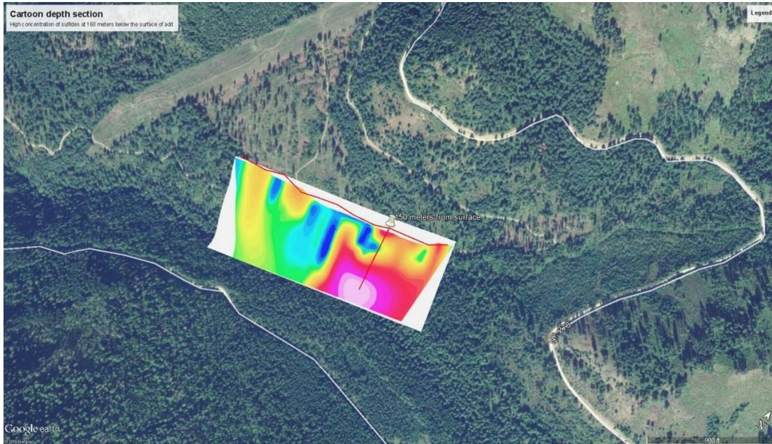
Figure 6) Above shows chargeability values in Google Earth – with pseudo depth section. The plot is a depth section of high chargeability values, with a very prominent anomaly in red. The picture above is intended to display the chargeability section below the survey line (in red).
