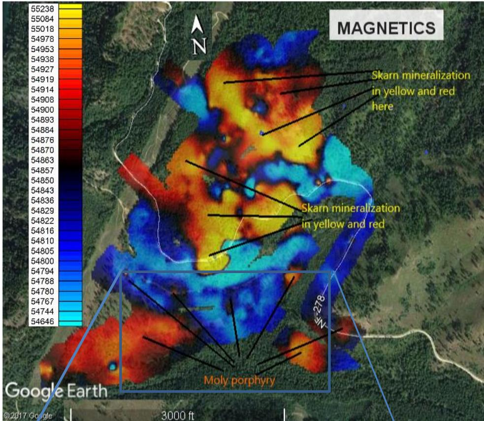
Figure 2) A hot-cold color display of magnetometer results, 2017. The “edges” of the complete survey area has been trimmed to focus on the core area. The hot-cold color plot highlights the core anomalies, however, some, “smaller” detail is sacrificed. Detail for smaller but significant features are shown in the inset below. NVH exhibits both large and small anomalies that are significantly related to high grade mineralization.
