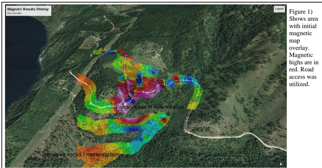
Figure 1) Shows area with initial magnetic map overlay. Magnetic highs are in red. Road access was utilized.
