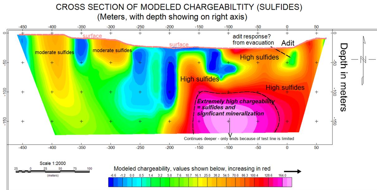
Figure 5) displays modeled chargeability. Red outlines the high values. Note extremely high values around -100 meters.
