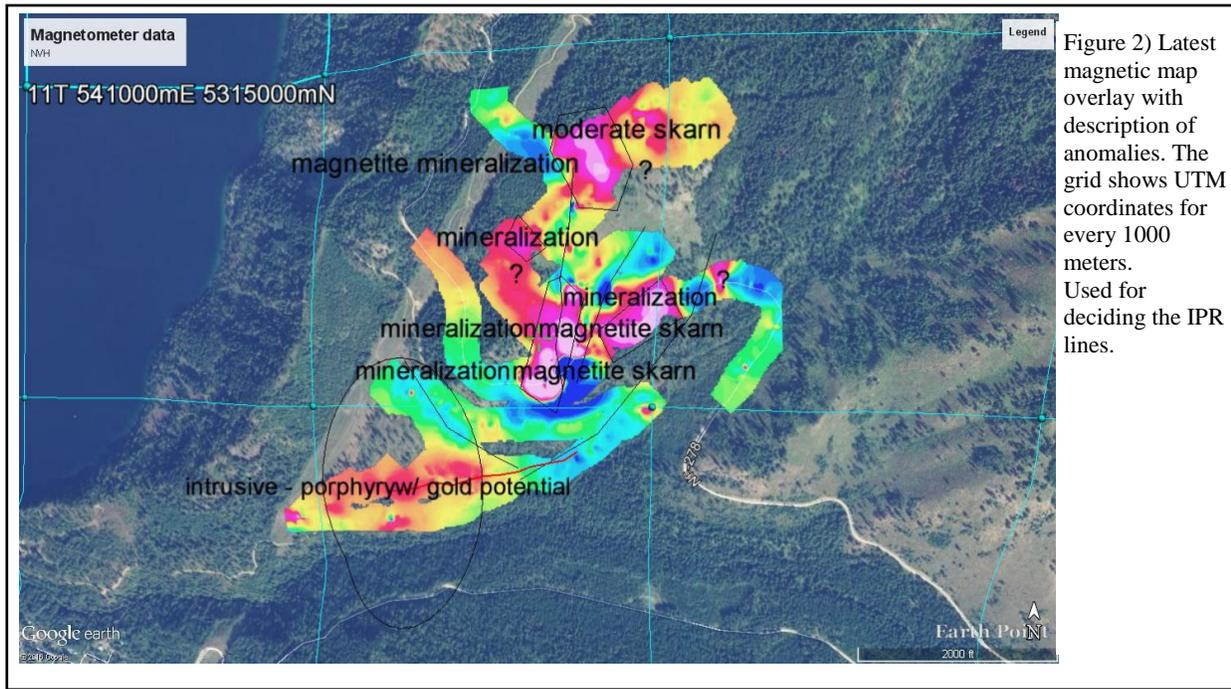
Figure 2) Latest magnetic map overlay with description of anomalies. The grid shows UTM coordinates for every 1000 meters. Used for deciding the IPR lines.
