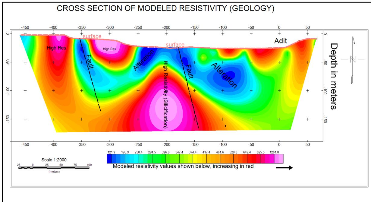
Figure 7) Modeled Resistivity section. Portrays high resistivity (silification in center) in red and faults with alteration zones. Note the close association of silicification to the west, and alteration near to top relative to the prominent chargeability high.
