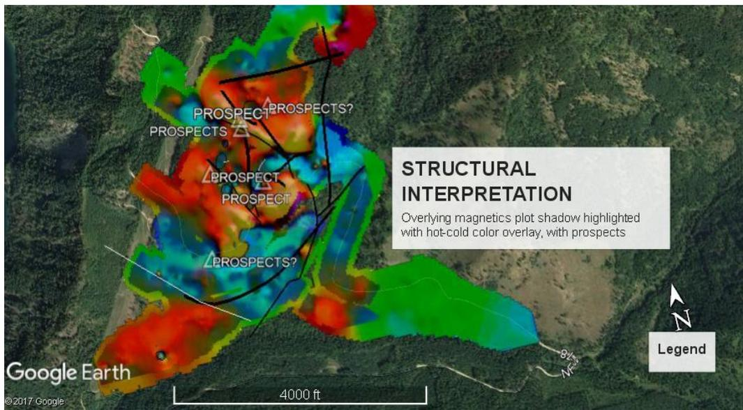
Figure 3) left depicts a combination of hot-cold color image of magnetics overlain on the normal color contour map for highlighting the major magnetic features, Fault lines (in black) primarily interpretive from the magnetics. General locations of Prospects (pits, not major adits) are shown based on observations. White line indicates probable separation of domains of intrusive rocks.
