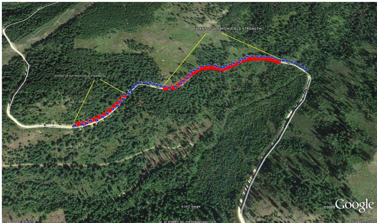
**Figure 6) Showing the area of VLF-EM anomalies in red, and location in blue flags. Total Field as recorded from 25.2 kHz, Jim Creek, Washington station. The red shows total field readings above 30 units and covers a large area.**
