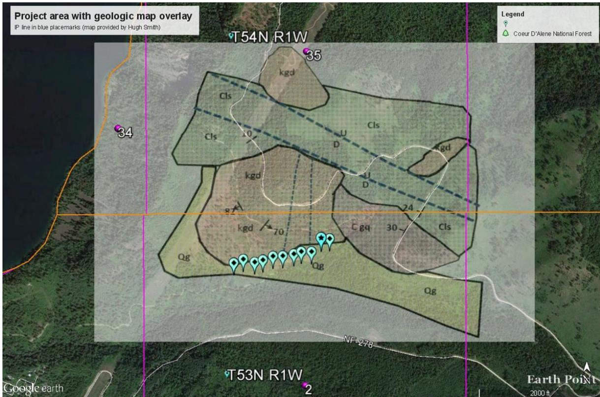
Figure 4) Location of stations and line of IPR survey over the Southwest target area. The underlying map shows the general geology of the area, The IPR line covered the Qg area but mapped lithologies of granodiorite and quartzites near the surface that extend below the Qg, alluvium plus.
