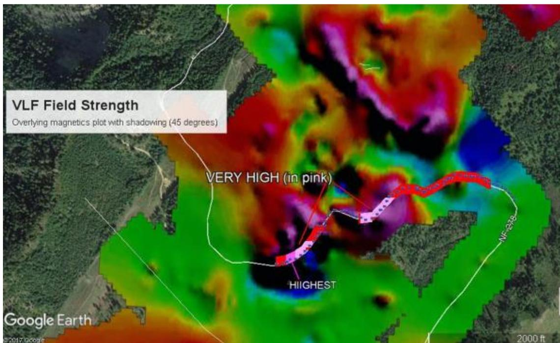
Figure 8) The VLF-EM results overlain over a color contour, shadow map of the magnetics. Note the VLF-EM highs correspond to the magnetic highs. The exception is at the eastern end. Here the VLF elevated readings denote alteration due to an intersection of faults.
