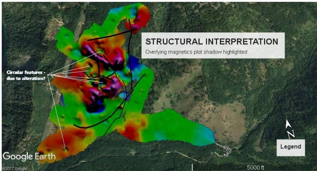
**Figure 5) Color contour - shadow image, magnetics, with interpreted faults (black lines), and circular features. Initial interpretation is supported by the field data, although features need confirmation by infill, as gridding can contour).**
