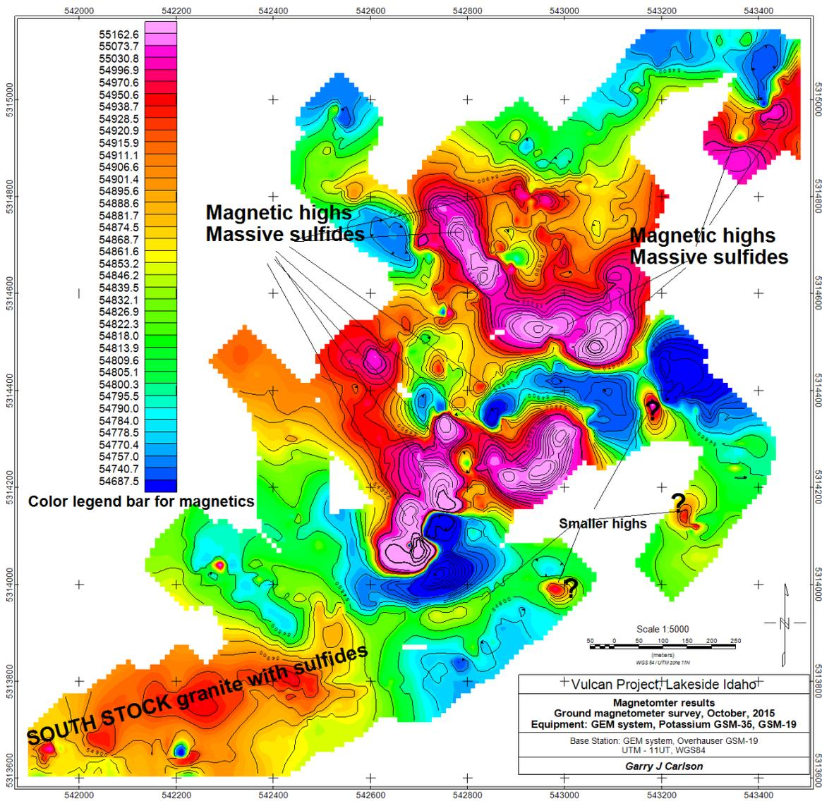
Figure 13) Shows the significant magnetic highs. Note the magnetic coverage is relatively limited and the extent of the highs can be further detailed with additional magnetometer lines.
