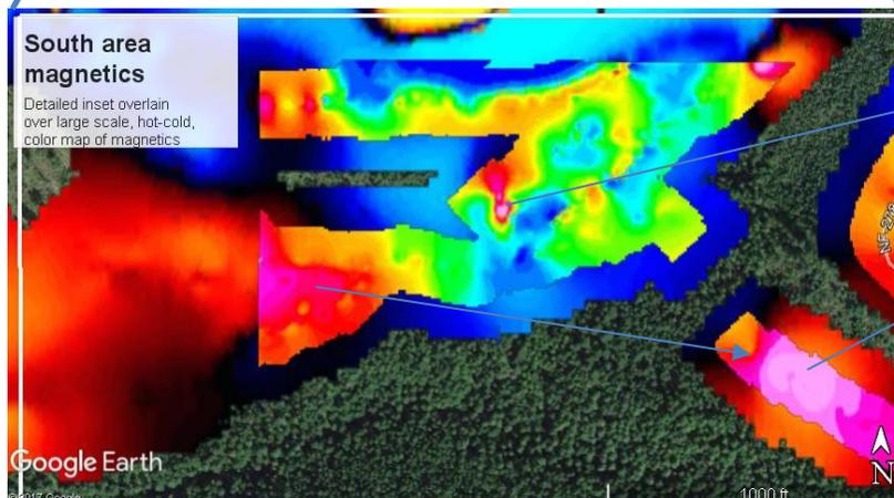
New anomaly 2017. Adit 3 with high grade moly mineralization shows a magnetic high.
