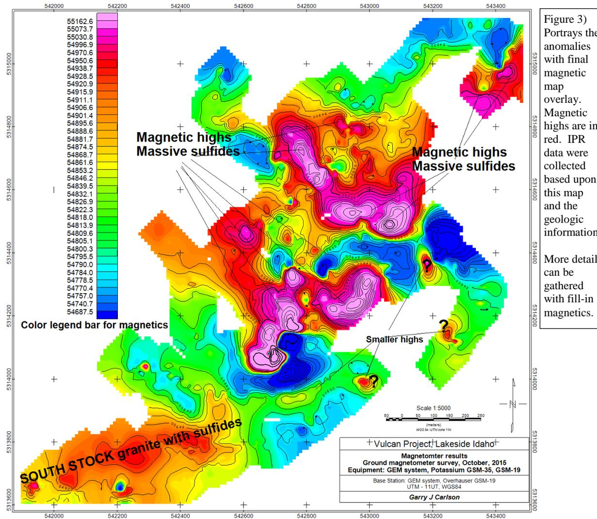
Figure 3) Portrays the anomalies with final magnetic map overlay. Magnetic highs are in red. IPR data were collected based upon this map and the geologic information. More detail can be gathered with fill-in magnetics.
