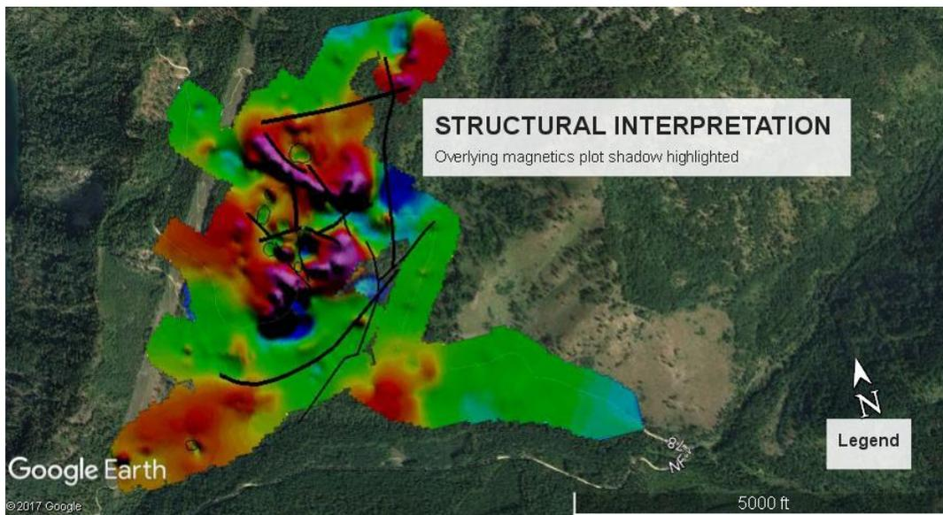
Figure 4) left showing the faulting in black and areas suggestive of solution breccias as evidenced by the circular features. The color contour map shows the highs (red) and lows (blue) and is enhanced by a shadowing, with a sun angle set at 45 degrees to the east and 60 degrees above the horizon.
