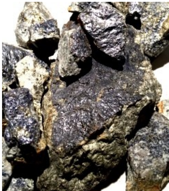
High grade Mo. Assaying with XRF 3.5% (not including gangue)
