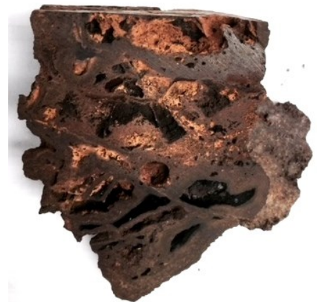
Evidence of massive sulfide skarn (Craig 2017). Dark bands contain Zn
